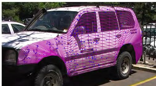
**Figure 8:** NURBS surface fitted to reconstructed object points.
